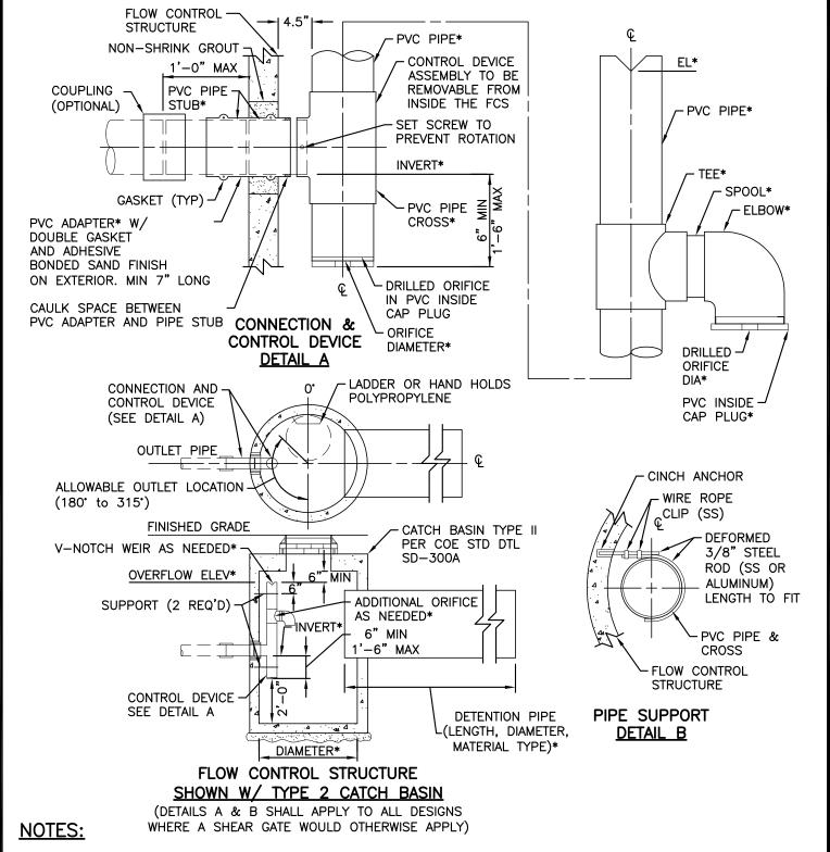
SPECIFIC DESIGN INFORMATION AS INDICATED ON APPROVED CONSTRUCTION DRAWINGS. INVERT OF DETENTION PIPE IN STRUCTURE SHALL BE EQUAL TO OR HIGHER THAN THE INVERT OF THE OUTLET PIPE. PRIVATELY-OWNED CONTROL STRUCTURES SHALL NOT BE PLACED IN CITY RIGHT-OF-WAY.
